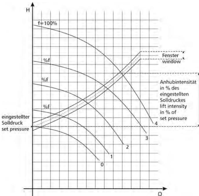
The Hydrovar can automatically compensate for system friction losses due to increased flow. Tables are available in most pump catalogues indicating the amount of friction loss that can be expected in various sizes of pumps at different flow rates. Use these tables to determine the friction loss for the pipe size you are using at maximum flow rate.
