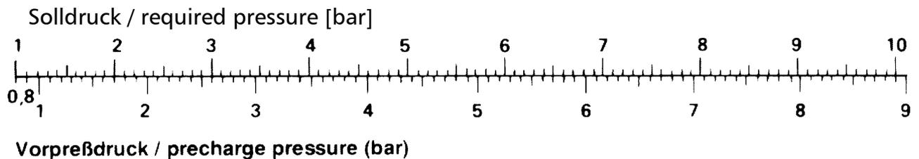
**Before checking the precharge pressure, take care, that the tank, is pressureless (no water inside).**
