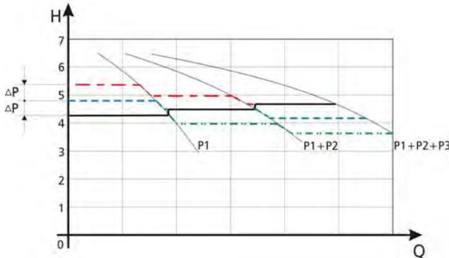
To do this, enter the amount of pressure drop you will allow before the next pump starts (=value of parameter ACTUAL VALUE DECREASE). The diagram shows the pressure drop and increase.
