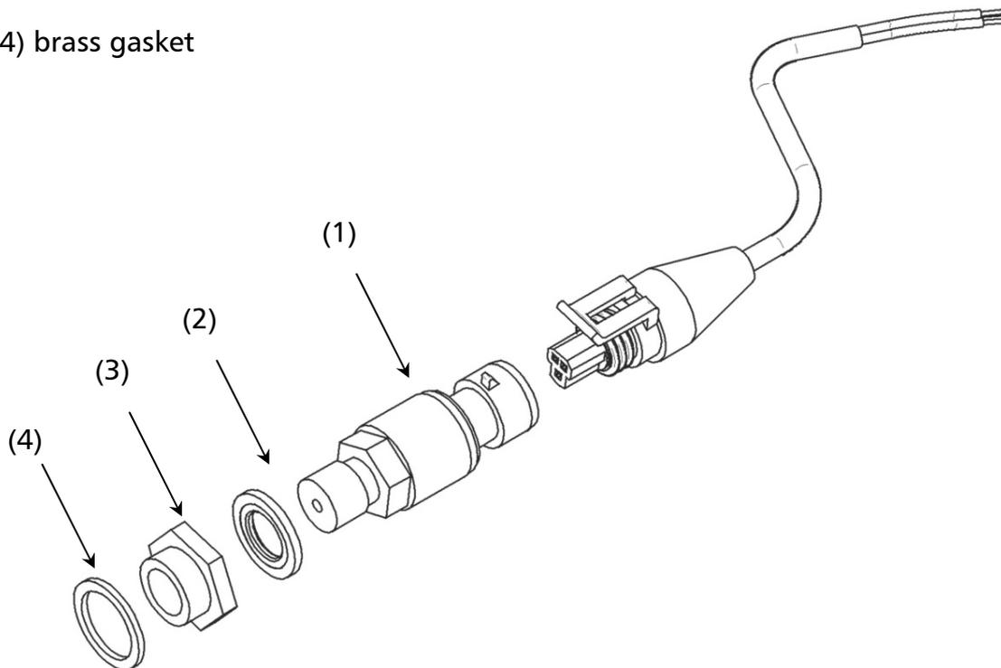
1. The transducer has an mechanical connection of G  $\frac{1}{4}''$ . If it is necessary put the reducer ( $\frac{3}{8}'' - \frac{1}{4}''$ ) into the pump or pipe by using included gaskets.
