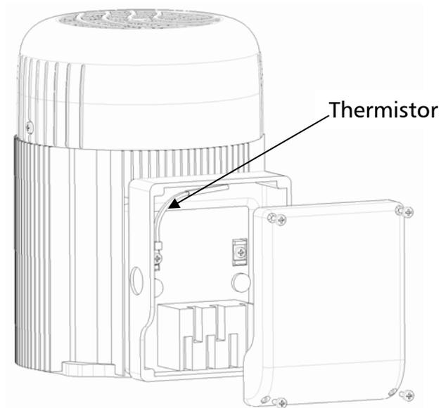
1. Open the cover of the conduit box and remove also the terminal block inside.
